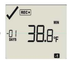
The logger will store and display 30 days of min/ max temperatures.
