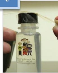
Put a piece of tape over the hole left from the probe and store the bottle safely until you get the data logger back.
