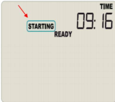
Press and hold the Start/Clear/Stop button. STARTING is displayed in addition to READY.
