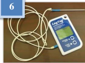
Attach the probe to the data logger and place both items into a padded envelope or small box with bubble wrap. **Complete the City of Chicago NIST Calibration RMA Form and include this form with the package.**
