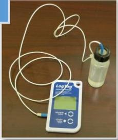
Stop the data logger. Remove the DDL, glycol bottle, and probe from your storage unit.
