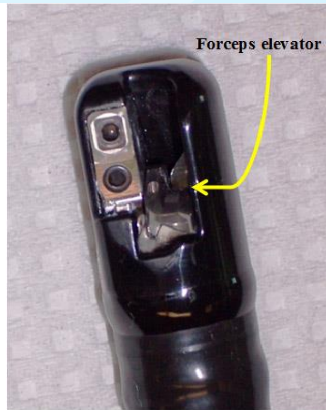
(b) Raised/ open forceps elevator
