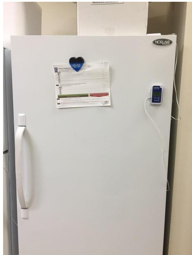
Place the data logger at eye level on the front of the storage unit next to your temperature log.
