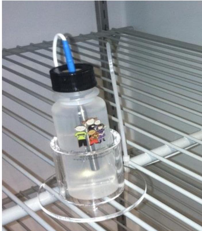
Place glycol bottle in the fridge/freezer for **at least 1.5 hours** prior to starting your logger to allow the solution to reach the appropriate temperature.
